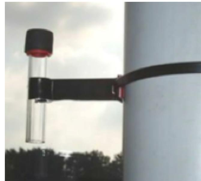
▲ Figure 2. Diffusion tube mounted on a lamp-post. (© Gradko)
