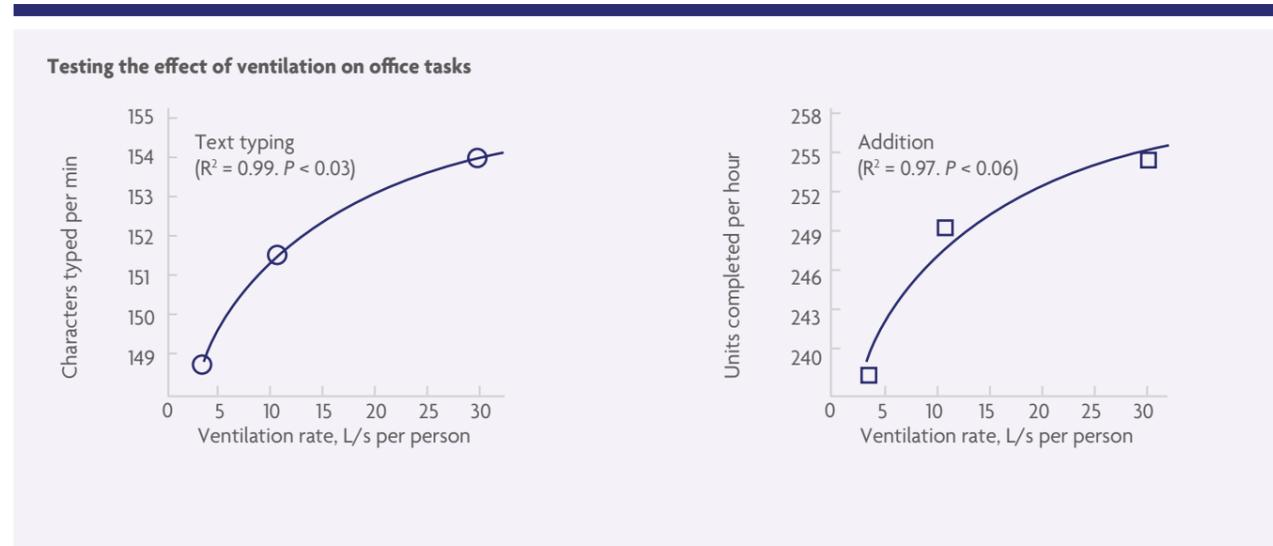
▲ Figure 3. Fresh air ventilation rate versus performance in an office environment.<sup>13</sup>
