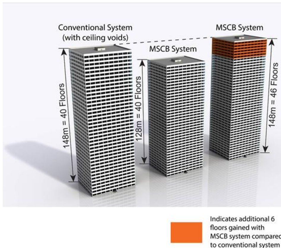
Figure 4. Building Heights and Floor Levels.
